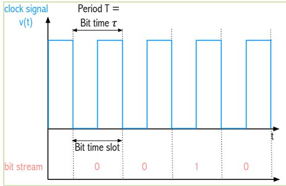
Fig. 1: Clock signal period and bit time
