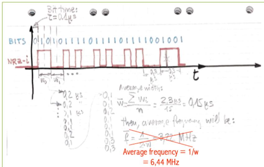
Fig. 2: NRZi data signal: Estimation of transmission frequency
