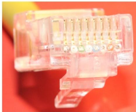
Fig. x. RJ-45 connector pin numbers (Front side)
