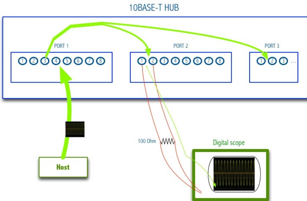
Fig. 2. Oscilloscope tracing a Differential Manchester signal from a 10BASE-T Hub
